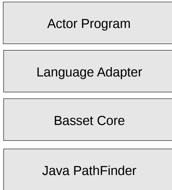
Figure 3.4: Basset systematic testing environment software layers
