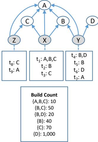
Fig. 1. An example dependency graph with build nodes A, B, C, and D; test nodes X, Y, and Z, actual dependencies for tests  $t_1$  through  $t_9$ , and the build count (number of times built) for sets of build nodes
