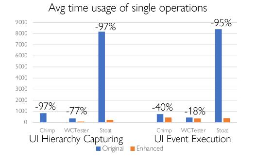
**TOLLER** substantially accelerates two types of operations
