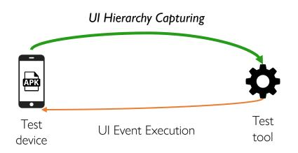
Obtain structured on-screen contents from the test device
