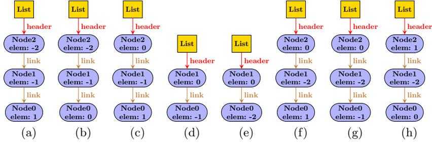
Fig. 2: First 8 solutions generated by the Alloy analyzer. For each structure, the square box is the list atom (*List*), and each ellipse is a node atom and is labeled with its identity (*Node0*, *Node1*, or *Node2*) and integer element (*elem*).
